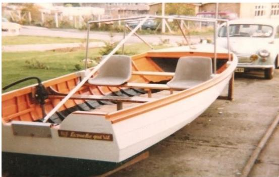
First things first, read up on clinker repairs, rivets, roves and how to bend wooden ribs and planks! But first where to buy sitka spruce. A setback, if they had any it was very expensive and some often reclaimed. I finished up with a 'mahogany' style flexible plank and cut to size oak ribs. Lucky I decided to paint inside and out. I removed the cabin and damaged wood. Surprising how many 'friends' visited and just shook their heads! If you haven't tried to steam
